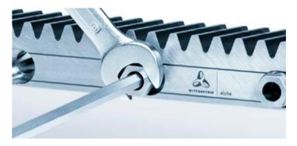
Previously, enormous effort was required to clamp racks to the mounting base using screw clamps. INIRA clamping integrates the clamping device in the rack. The rack incorporates a mounting sleeve which is guided over the head of the fastening screw to ensure quick and ergonomic clamping.
