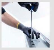
The assembly bushing and the mounting pin are turned in opposite directions until the bushing engages in the pin bore and then pushed in by hand up to the second marking.
